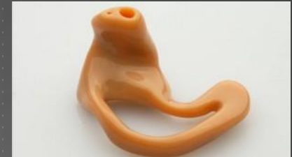
Hearing aid created from 3D printed mold
