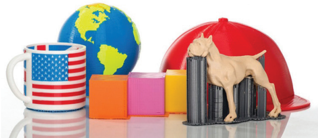
Figure 10: Typical "multi-color" parts from FDM
